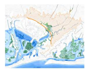
A storm surge barrier protecting the airport and the surrounding community by linking to high ground to the north and south of the bay would be 6.7 miles long and protect an area of 21.5 miles<sup>2</sup>.
