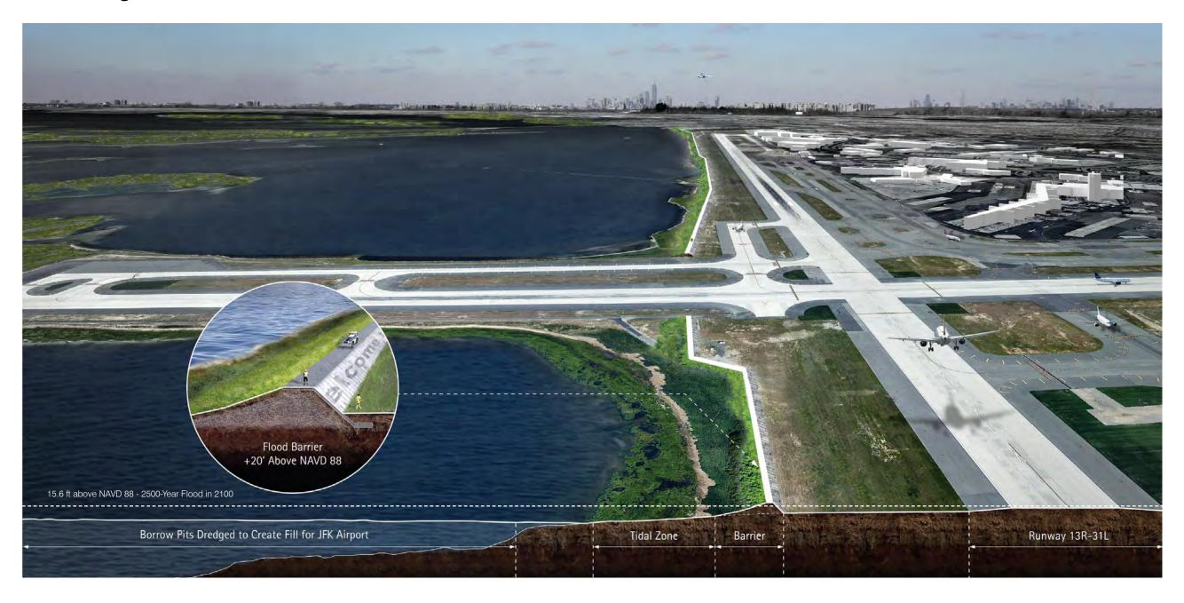
The storm surge barrier is designed so its top surface reaches 20 feet above NAVD 88. It would operate during more intense, less frequent storms. At JFK Airport, the barrier would need to remain open to allow access to the runways. During an
