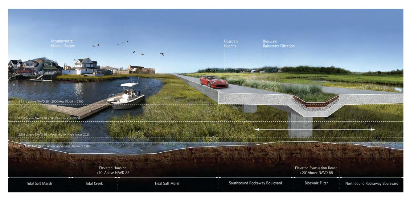
The length of Rockaway Boulevard and Rockaway Turnpike spanning the floodway could be elevated to create an evacuation route that would remain passable during any flood event. Over time, the commercial lots surrounding the raised causeway
