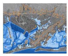
A tidal barrier directly following the shoreline would be extremely long relative to the area it could potentially protect. It would be the most costly to build and the most difficult to maintain under sea level rise.
