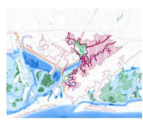
A tidal barrier following the Rockaway Turnpike would protect a large area with a relatively short barrier. However, it would require multiple closure structures or, if passive, would cause extensive damage to Idlewild Marsh and the surrounding waterways.
