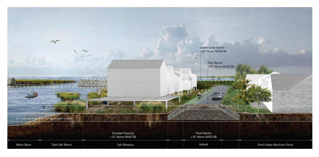
The tidal barrier is designed to a height of 10 feet above NAVD 88 along its top surface. The barrier follows the path of existing roads, so it could be built on public land and provide a means of upgrading transportation infrastructure. This protective measure would be passive, so it would
