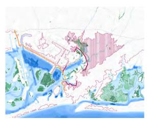
A tidal barrier following the first continuous inland roads would be relatively short in length and could protect a significant area from tidal flooding and minor storm events. This barrier could operate passively without causing damage to the existing marshes.
